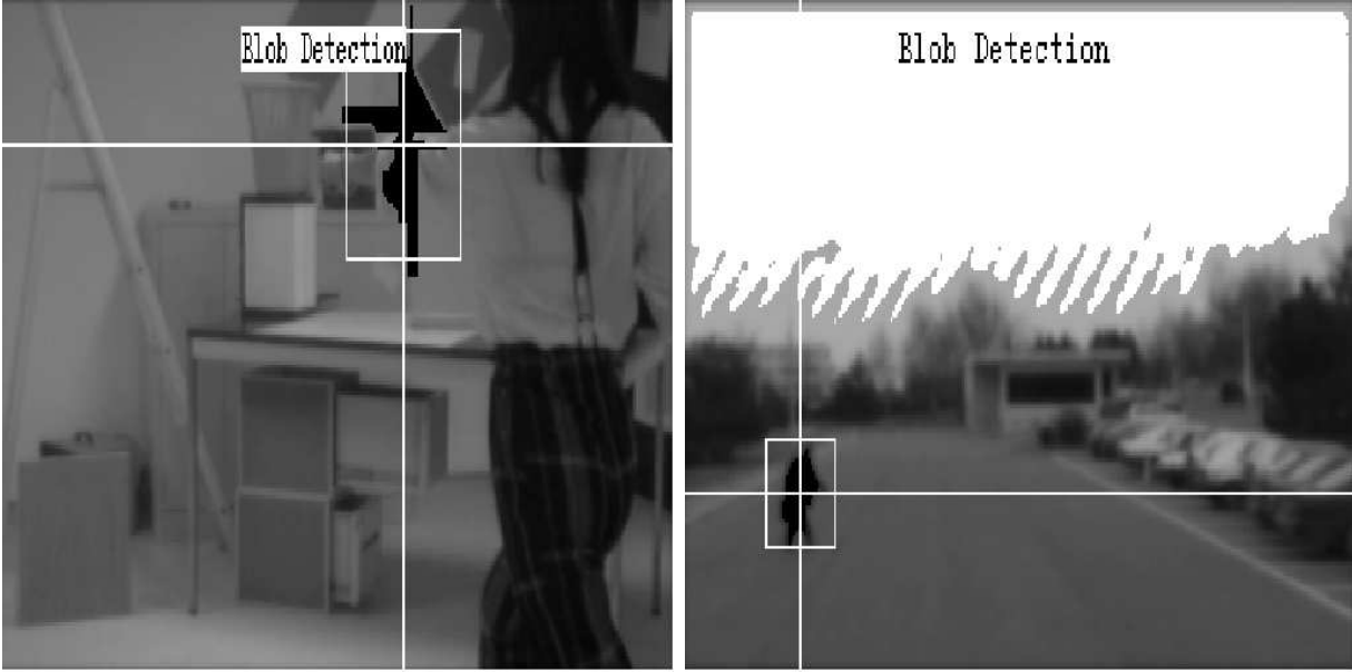
Figure 13: Two examples of target detection. The arm of the Kung-Fu teacher in the left view, and the pedestrian in the right view have been detected as the most important object to focus on, in the scene. Both objects correspond to regions for which residual disparity is maximal. This is consistent with what could be expected, from a naive observation.
