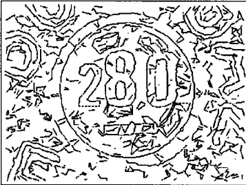
Fig. 4. Set of edgels obtained with no noise elimination.
