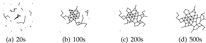
Fig. 12. Evolution of node's position and associated graph depending on time. In this simulation there is 50 nodes with a range of 10 on a square of 100 \times 100 . Nodes are not connected at the beginning of simulation
