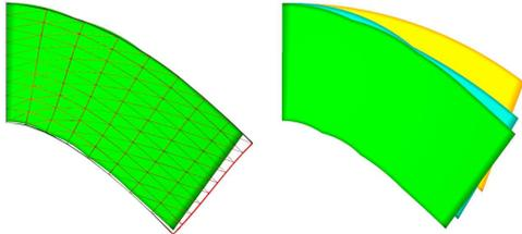
Fig. 6. Left: comparison of our model (green) with 5 frames along the main axis and  $10 \times 10 \times 9$  samples in the volume, with a St-Venant-Kirchhoff model (red) with  $10 \times 10 \times 9$  points, with same loads and material parameters. Right: comparison of beams with 5, 3 and 2 frames in our model, from front to back.
