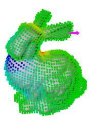
Fig. 4. Sample points in a deformed configuration with hue mapping of the strain (hi res. bunny example: 15000 samples, 2 frames)
