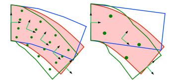
Fig. 10. Comparison of FEM simulation (in blue) and frame-based simulation (in green) for  $4 \times 4 \times 4$  (left) and  $2 \times 2 \times 2$  (right) FEM nodes and integration points. The reference high-resolution FEM is shown in red. The integration points are shown as disks. The green curve is the outline of a visual model bound to the frames.
