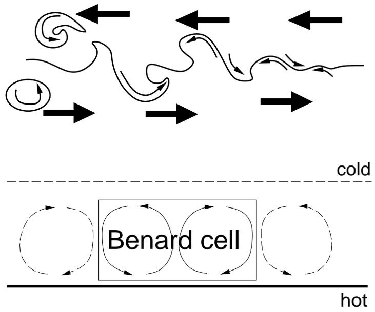
Figure 1: Some macroscopic structures in fluid motions.
