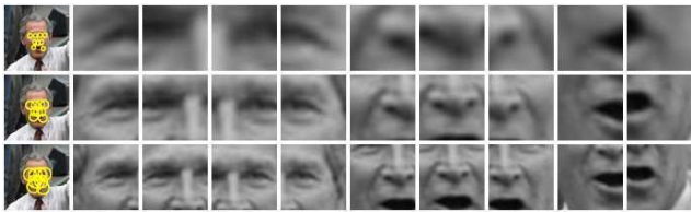
Fig. 5 Illustration of our SIFT-based face descriptor. SIFT features (128D) are extracted at 9 locations and 3 scales. Each row represents a scale at which the patches are extracted: the top row is scale 1, the middle row is scale 2 and the bottom row is scale 3. The first column shows the locations of the facial features, and the remaining nine columns show the corresponding patches on which 128D SIFT descriptors are computed. The descriptor is the concatenation of these 3 \times 9 SIFT features.
