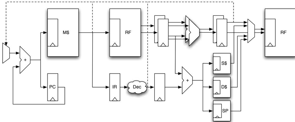
■ **Figure 1** Pipeline of Patmos with fetch, decode, execute, and memory/write back stages.
