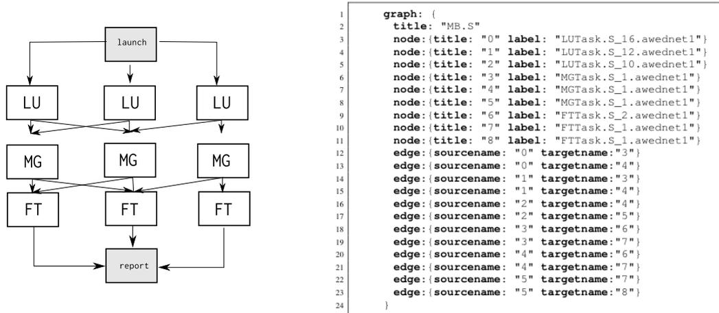
Fig. 6. Pattern (left) and topology definition (right) used in NASGrid
