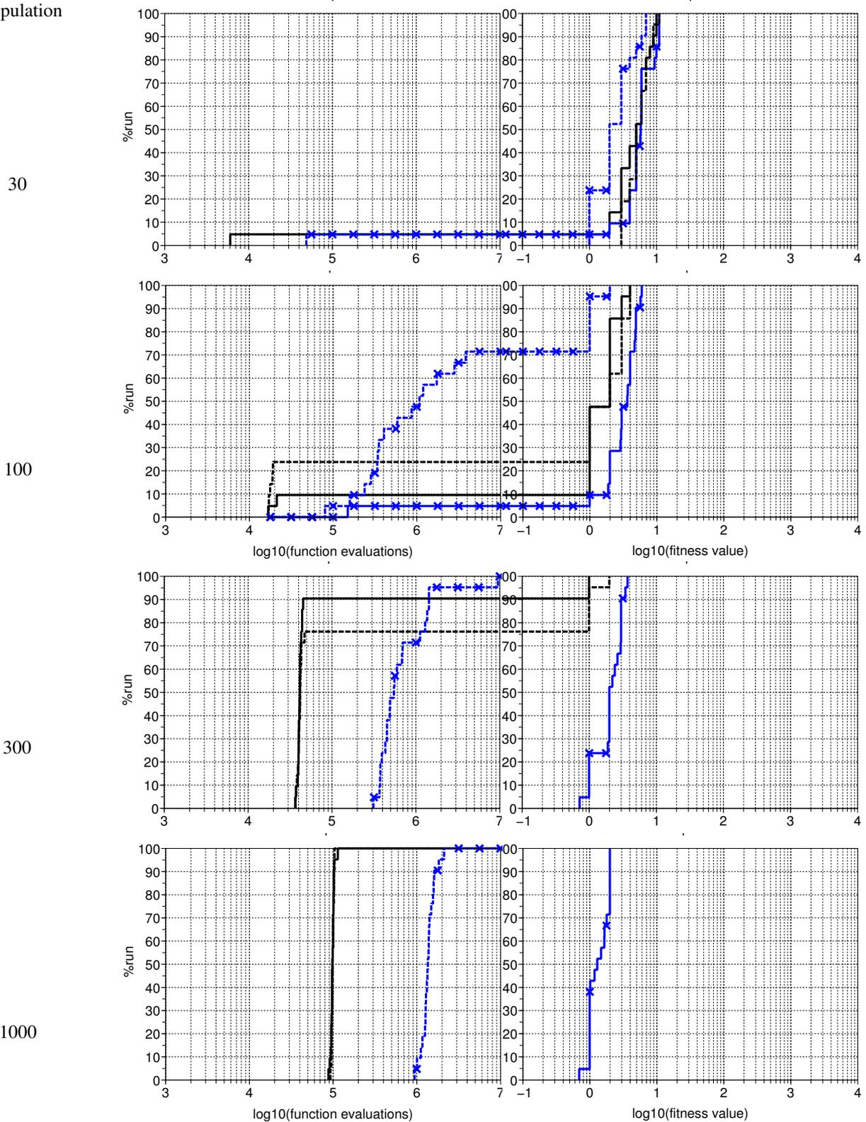
Figure 10: Rastrigin function in 10-D: empirical cumulative distribution (ECDF) of the number of function evaluations to reach the target function value  $10^{-9}$  (left column) and ECDF of the best function value after the maximum number of function evaluations is exceeded (right column). Swarm/population size of 30, 100, 300, 1000 from top to bottom. s-PSO with small crosses, CMA-ES without; solid lines: rotated, dashed lines: non-rotated function.
