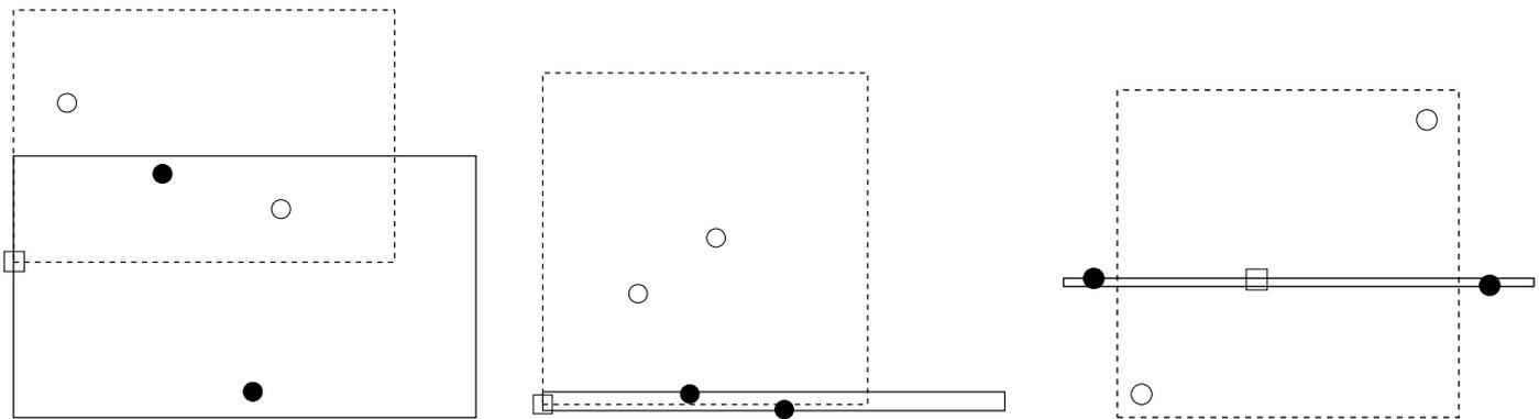
Figure 1: Domain of non-zero density for the intermediate particle position  $\mathbf{x}^{t+\frac{1}{2}} = \mathbf{x}^{t+1} - w(\mathbf{x}^t - \mathbf{x}^{t-1})$ , in three cases (solid rectangles), and after a  $45^\circ$  rotation around  $\square$  (dashed rectangles). The symbols indicate:  $\square$  = particle  $\mathbf{x}^t$ ,  $\bullet$  =  $\mathbf{p}$  and  $\mathbf{g}$  (interchangeably),  $\circ$  =  $\mathbf{p}$  and  $\mathbf{g}$  in the rotated case.
