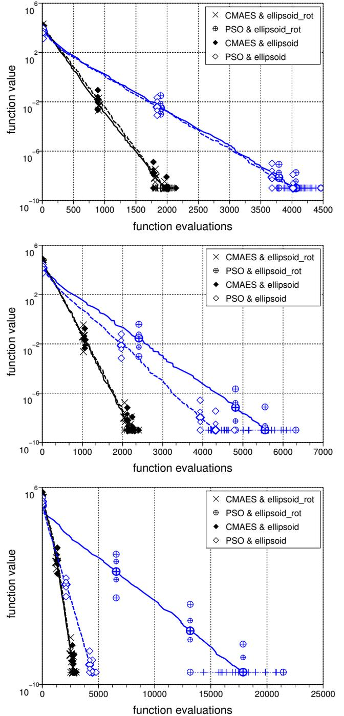
Figure 2: Ellipsoid function in 10-D: time evolution of the median function value with a function condition number  $\alpha$  of 1 (top), 10 (middle), and 100 (bottom). Small symbols indicate the 25% and 75%-ile, large symbols indicate smallest and largest value from 21 trials. Solid lines: rotated function, dashed lines: non-rotated (separable) function. s-PSO:  $\oplus$ ,  $\diamond$ ; CMA-ES:  $\times$ ,  $\blacklozenge$
