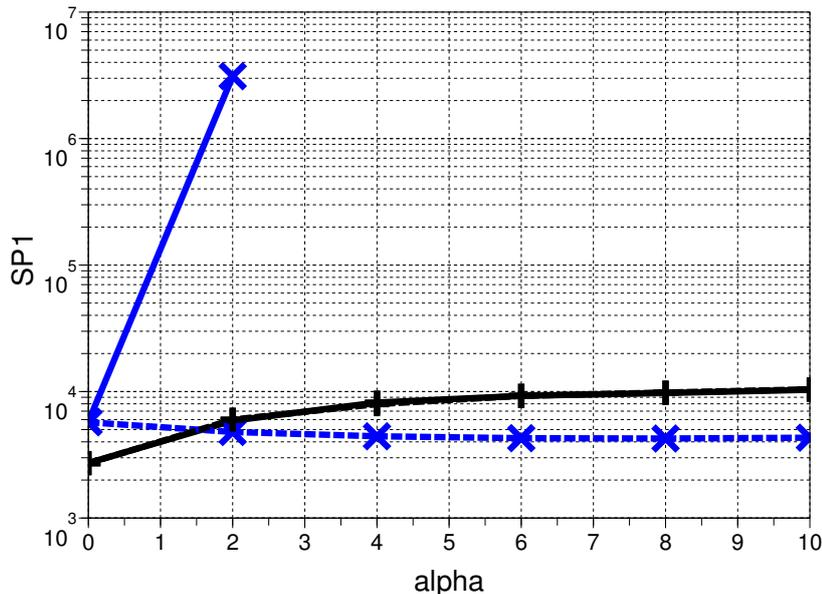
Figure 8: Diff-Powers function in 10-D:  $\widehat{SP1}$  (number of function evaluations) versus parameter  $\alpha$ . s-PSO:  $\times$ , CMA-ES:  $+$ ; solid lines: rotated, dashed lines: non-rotated function. For CMA-ES both graphs are virtually identical. Missing points indicate that  $10^7$  function evaluations were exceeded in all trials. The axis parallel function becomes with increasing  $\alpha$  even more easy to solve for s-PSO.
