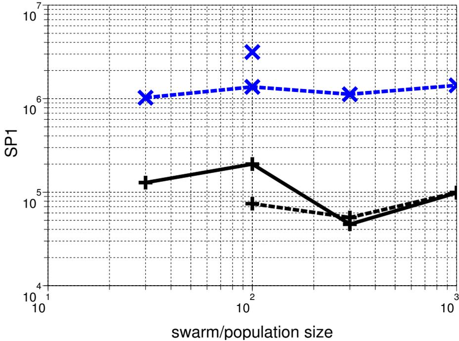
Figure 11: Rastrigin function in 10-D:  $\widehat{SP1}$  (number of function evaluations) versus swarm size/population size. s-PSO:  $\times$  (above lines), CMA-ES:  $+$  (below lines); solid lines: rotated, dashed lines: non-rotated function. For missing points no trial reached the target function value.  $\widehat{SP1}$  shows comparatively flat graphs, because the number of function evaluations to reach the target value in successful trials is negatively correlated with the success rate.
