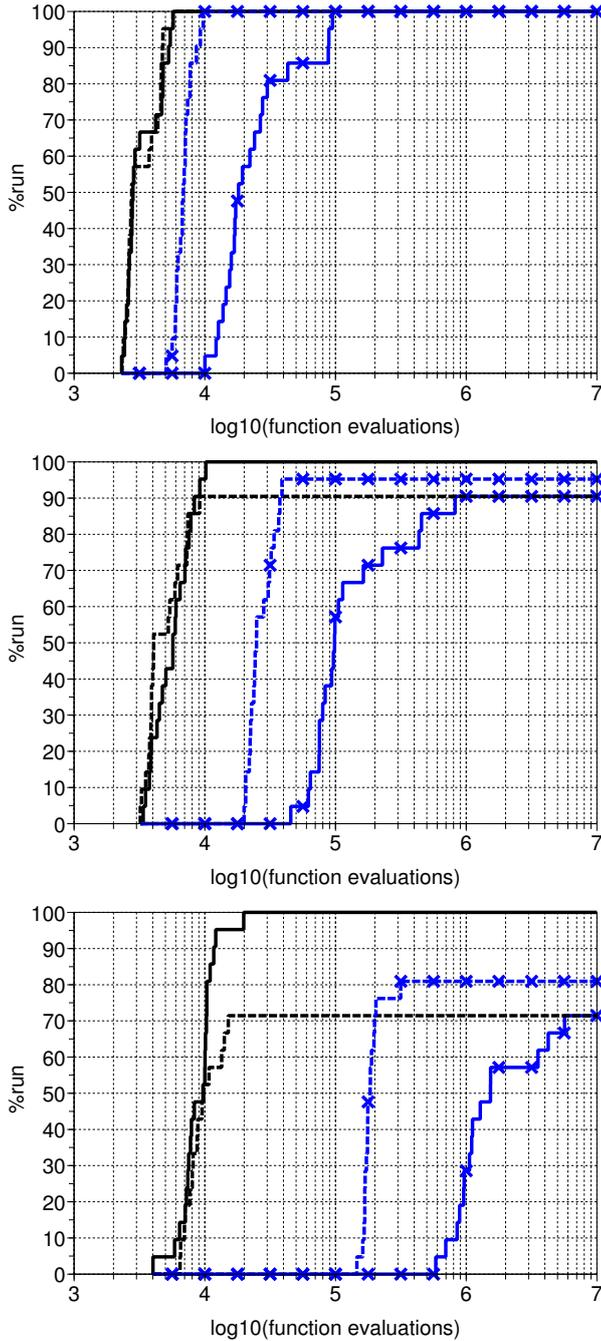
Figure 5: Rosenbrock function in 10-D: empirical cumulative distribution of the number of function evaluations to reach the target function value with a function conditioning parameter  $\alpha$  of 1 (top), 10 (middle), and 100 (bottom). s-PSO (with small crosses) corresponds to the two lines to the right in each case. Solid lines: rotated, dashed lines: non-rotated function.
