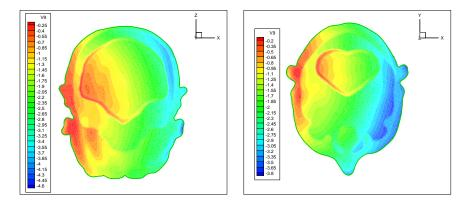
Figure 8: Calculations with the DGTD- $\mathbb{P}_1$  method. Mesh M3: contour lines of local SAR over maximum local SAR in log scale (selected cut planes).
