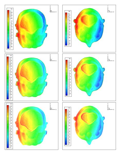
Figure 6: Calculations with the DGTD- $\mathbb{P}_1$  (top), DGTD- $\mathbb{P}_2$  (middle) and DGTD- $\mathbb{P}_3$  (bottom) methods. Mesh M1: contour lines of local SAR over maximum local SAR in log scale (selected cut planes).
