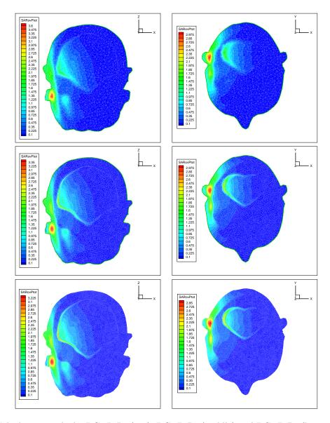
Figure 7: Calculations with the DGTD- $\mathbb{P}_1$  (top), DGTD- $\mathbb{P}_2$  (middle) and DGTD- $\mathbb{P}_3$  (bottom) methods. Mesh M1: contour lines of normalized local SAR (selected cut planes).
