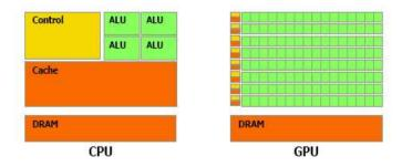
Figure 1: GPU vs CPU design philosophies.
