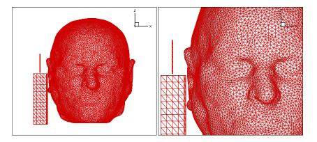
Figure 4: Simplified mobile phone model and its positioning.
