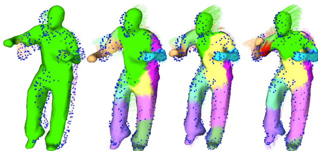
Figure 1. Convergence of the method in fitting frame 30 of Lock sequence (courtesy U. Surrey [15]), using frame 20 as reference (left). Target observation points are shown in blue, color lines show probabilistic associations from observations to reference vertices. The method estimates rigid clusters coherent with both the spatial and motion characteristics of the model, in particular recovering the correct partition and motion of arm and forearm.
