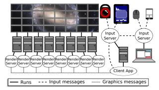
Figure 2. Example jBricks configuration: wall's graphics client and input server for motion tracker and tablet run on client node; input server for mouse, keyboard and smartphone run on user's laptop.
