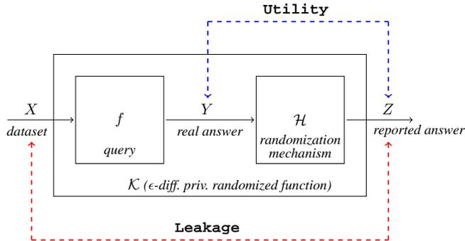
**Fig. 2.** Leakage and utility for oblivious mechanisms
