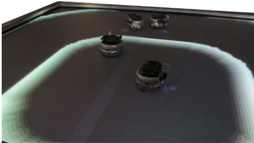
Fig. 7. Snapshot of an experiment using the Khepera robots on the interactive ROMEA table. The experiment uses a circular neighborhood with radius 2.5 and M=6
