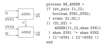
FIG. 8 – A weakly endochronous version of ADDER.
