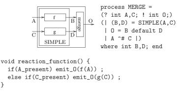
FIG. 5 – Extending SIMPLE with a shared resource. Dataflow (top left), Signal code (top right), single-loop implementation (bottom). The driver is that of Fig. 3.
