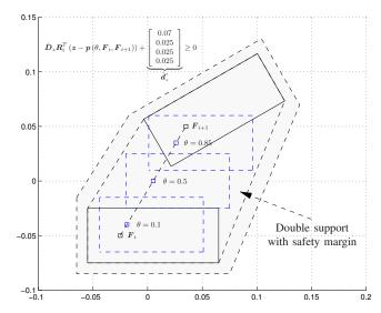
Fig. 2. Approximation of the constraints on the ZMP when in double support. The polygon depicted in gray represents the double support constraints without safety margin. The approximating constraints (in blue dashed line) have tighter safety margin compared to the normal single support constraints.
