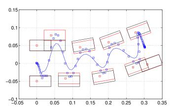
Fig. 3. Motion generation when using formulation (18) with  $\mu = 2000000$ .
