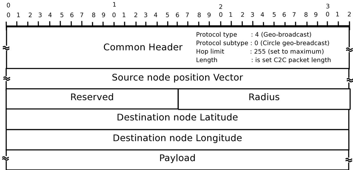
Figure 3: Geo-broadcast packet
