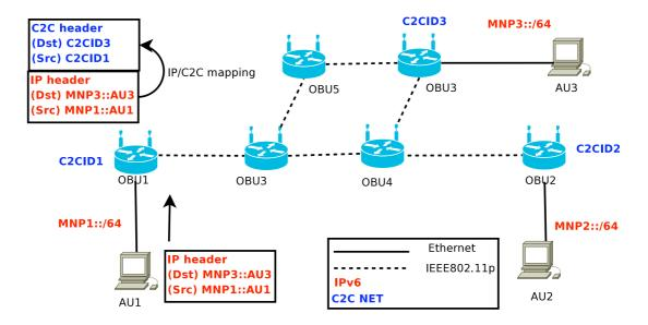
Figure 6: in-vehicle network discovery
