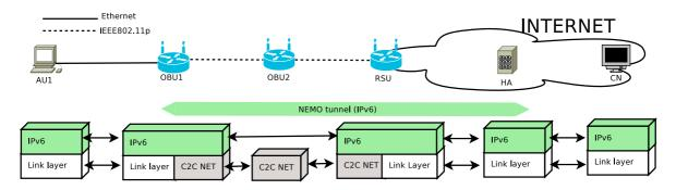
Figure 5: V2I Geo-Unicast Scenario
