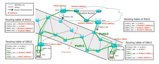
Figure 27: Using alternative route between OBU and CR (Scenario 3)
