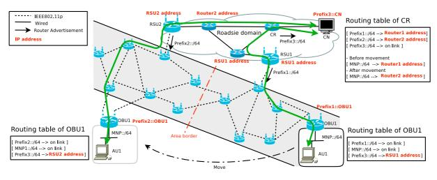
Figure 26: Using alternative route between OBU and CR (Scenario 1)
