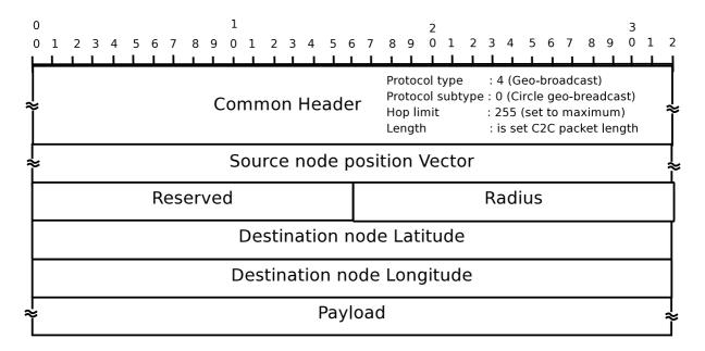
Figure 3: Geo-broadcast packet
