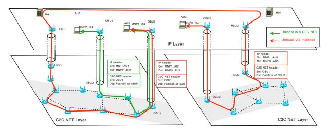
Figure 11: Unicast Over C2C NET
