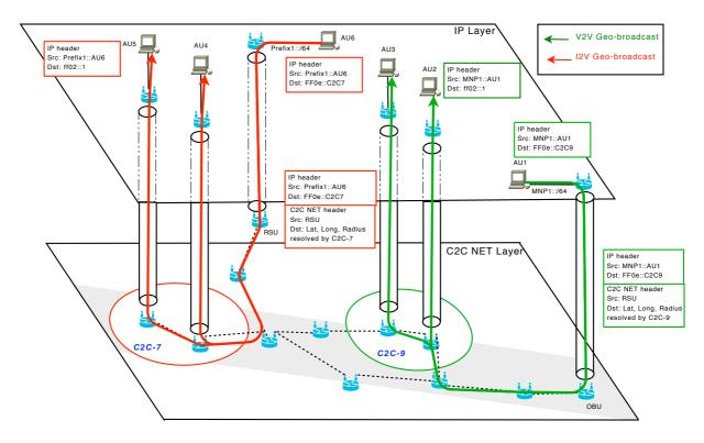
Figure 17: Multicast over Geo-Broadcast
