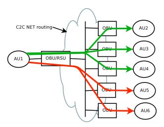
Figure 15: IP model on Geo-Broadcast
