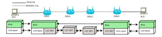
Figure 4: V2V Geo-Unicast Scenario
