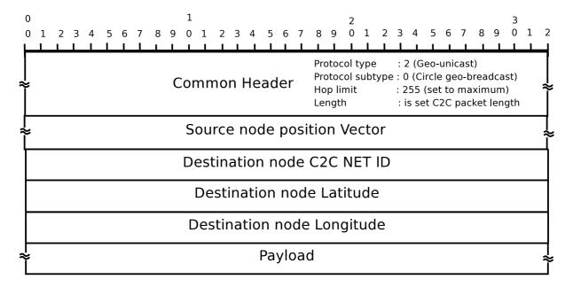
Figure 2: Geo-unicast packet
