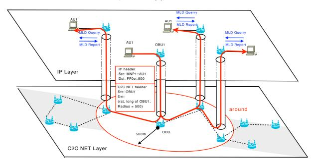
Figure 14: Multicast Over Around Geo-Broadcast
