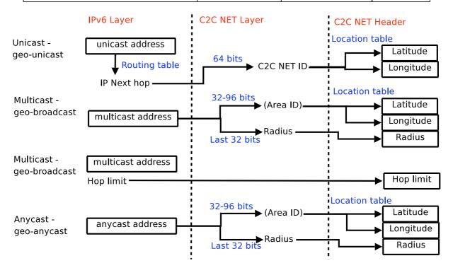
Figure 10: Service Access Point between IPv6 and C2C NET
