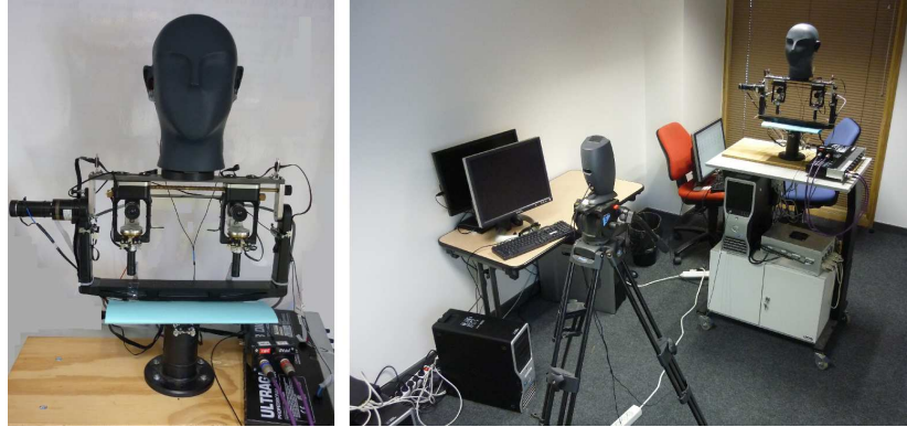
Figure 1: A binaural dummy head is placed onto a robotic head which can perform precise and reproducible pan and tilt motions (left). The emitter (a loud-speaker) is placed in front of the robot at approximately 2.7 meters (right).
