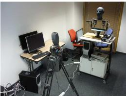
Figure 1: A binaural dummy head is placed onto a robotic head which can perform precise and reproducible pan and tilt motions (left). The emitter (a loud-speaker) is placed in front of the robot at approximately 2.7 meters (right).
