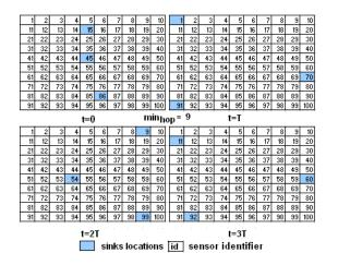
Fig. 4. The sinks locations pattern in 10x10 grid network (L = 10)
