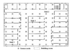
Fig. 1. 10x10 grid of cells with sensors in office building (L=10)
