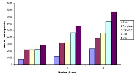
Fig. 5. Network lifetime with 100 sensors (10x10 grid)
