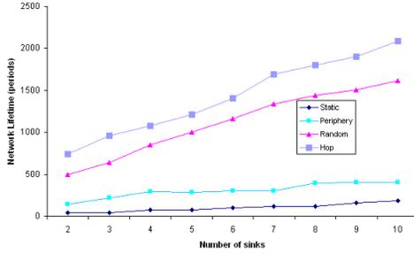
Fig. 6. Network lifetime with increasing number of sinks
