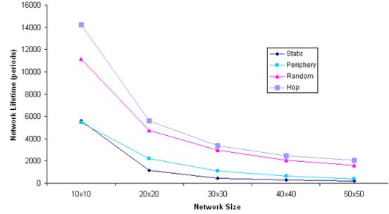
Fig. 8. Network lifetime with increasing network size
