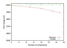
FIGURE 18. The Remora-based implementation does not impose additional CPU overhead compared to the Contiki-based implementation.
