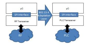
Figure 3: Emulation of a classic RF transceiver by a PLC transceiver trough an enhanced SPI interface
