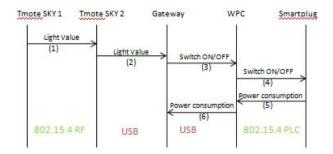
Figure 10: IEEE 802.15.4 frames exchange diagramm
