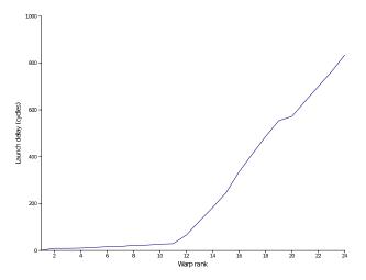
Fig. 2. Launch delay in respect of warp rank
