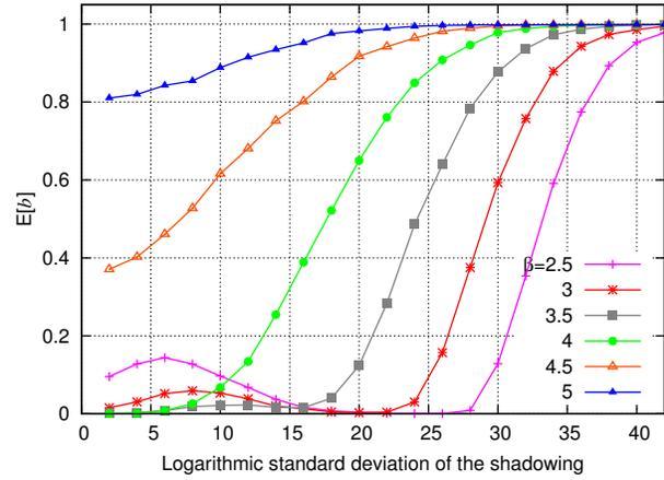
(b) OFDMA, 23.1 Erlang per km<sup>2</sup>Fig. 3. Blocking probability for OFDMA network as on Figure 2 with traffic 34.6 Erlang per km<sup>2</sup> and 23.1 Erlang per km<sup>2</sup>.
