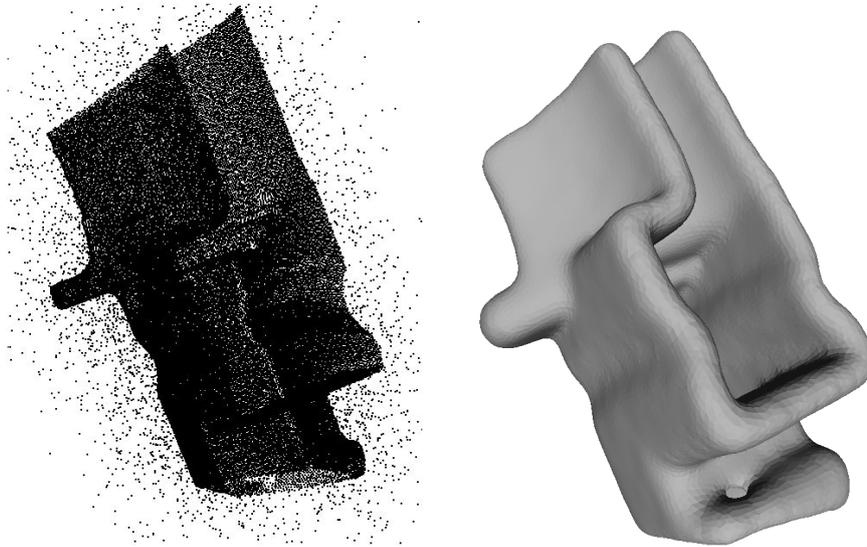
Figure 2: **Left:** A three-dimensional set of points uniformly sampled on the surface of a mechanical part to which 10% of points sampled uniformly at random in a box enclosing the mechanical part have been added. **Right:** An isosurface of the distance function  $d_{\mu, m_0}$  to the empirical measure based on the observations. This isosurface successfully recovers the topology of the mechanical part. In this example,  $m_0 = 0.003$ .
