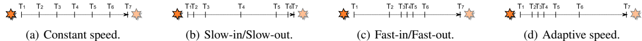
Figure 1. Different temporal distortion strategies for animated transitions. Solid shapes show original positions, faded shapes show ending positions.
