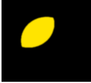
Fig. 8. Chopped pupil amplitude as a result of two aperture with 25% overlap. The overlap region shows the permitted light.
