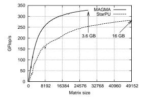
Figure 5. SGETRF with MAGMA and StarPU
