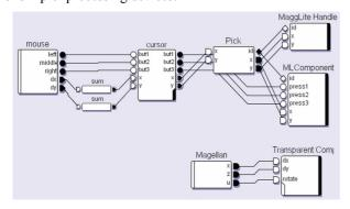
Figure 10: A possible interaction-graph (described by an ICon configuration) for the scene-graph of Figure 7.
