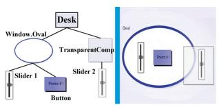
Figure 7: A simple MaggLite scene-graph and the corresponding interface.
