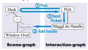
Figure 12: Mixed-graphs – Responsive Handle. Pick receives signals, and queries for picked objects (1). It transmits values to the handles device (2) which inserts a handle object in the scene-graph (3).
