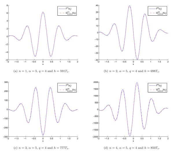
Figure 3: The exact values of  $f_1^{(n)}(x_i)$  and the estimated values  $D_{h,\alpha,\alpha,q}^{(n)}f_1(x_i)$  for  $\delta=0.15$ .
