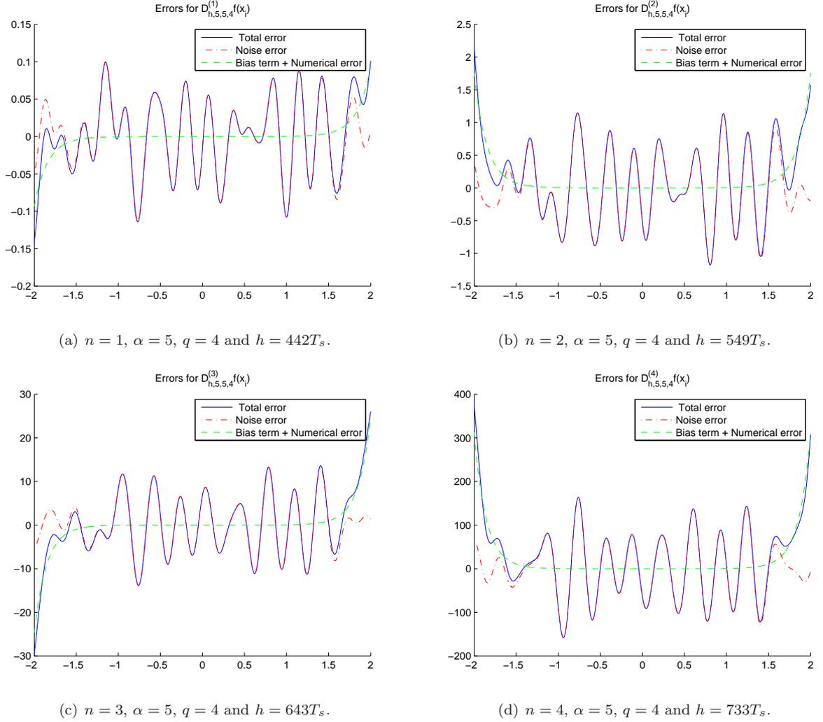
Figure 5: The estimation errors for the estimated values  $D_{h,\alpha,\alpha,q}^{(n)} f_2(x_i)$  for  $\delta = 0.15$ .
