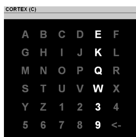
Figure 1: A 6x6 P300 speller. The application highlights in a random order columns and rows. The user looks at the desired letter. When the letter is highlighted, a P300 is generated. Detecting this specific transient event, it is possible to know which letter is requested.
