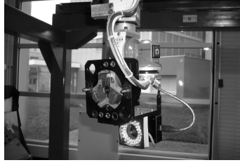
Fig. 5.8 Camera and light-ring mounted on the robot end-effector.
