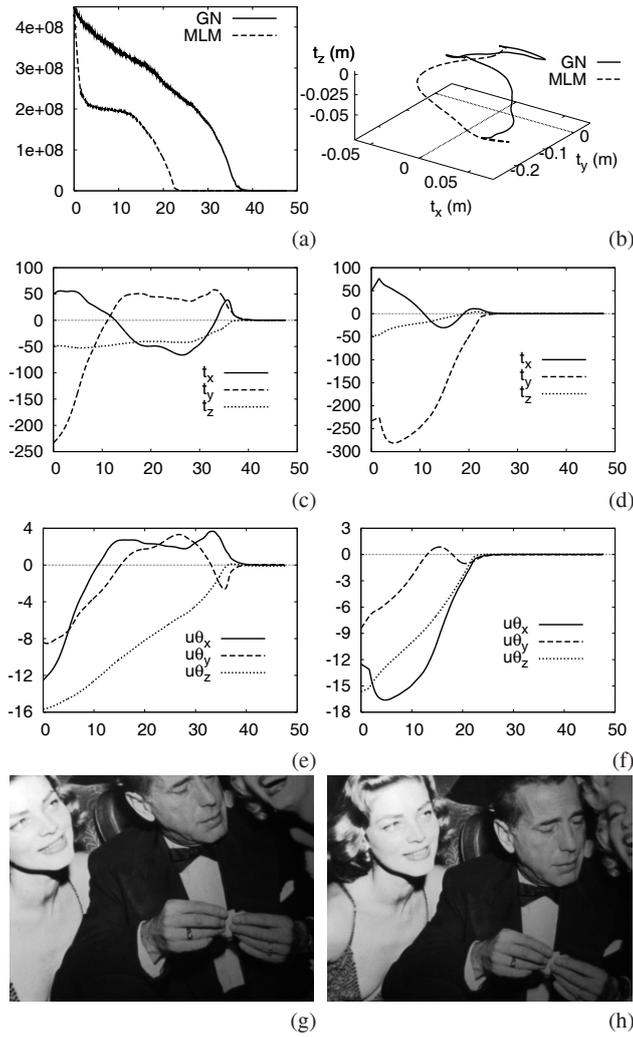
**Fig. 5.3** First experiment, MLM versus GN method ( $x$  axis in seconds): (a) comparison of cost functions; (b) comparison of camera trajectories; (c) translation error for the GN method (in mm); (d) translation error for the MLM method (in mm); (e) rotation error for the GN method (in deg); (f) rotation error for the MLM method (in deg); (g) initial image; and (h) final image.
