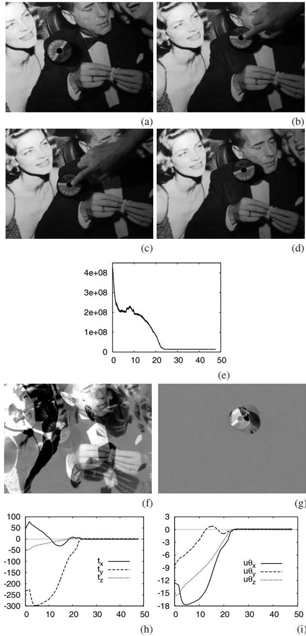
**Fig. 5.5** Third experiment, occlusions ( $x$  axis in seconds): (a) initial image; (b) image at  $t \approx 11$  s; (c) image at  $t \approx 13$  s; (d) final image; (e) cost function; (f)  $\mathbf{I} - \mathbf{I}^*$  at the initial position; (g)  $\mathbf{I} - \mathbf{I}^*$  at the end of the motion; (h) translation errors (in mm); and (i) rotation errors (in deg).
