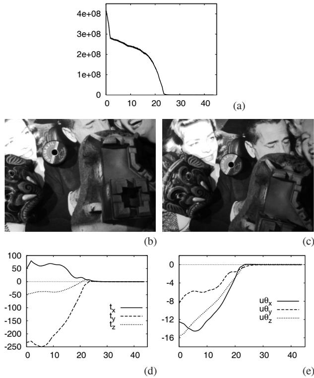
**Fig. 5.7** Fourth experiment, robustness with respect to depths ( $x$  axis in seconds): (a) cost function; (b) initial image; (c) final image; (d) translation errors (in mm); and (e) rotation errors (in deg).
