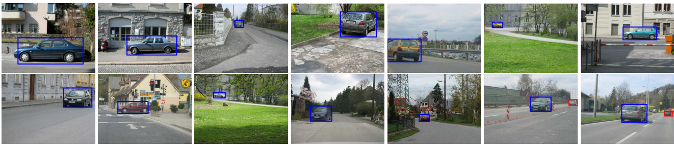
Figure 5. Successful detections on the PASCAL VOC 2005 Cars Test 1. The last two images in the bottom row show correct detections (small red rectangles) showing up as false positives because they were not annotated in the dataset. Please view in color.
