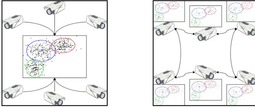
Figure 1: Central and Distributed System, (*left* a central system, where all cameras send their observations to a single computer which learns a certain model, and (*right*) a distributed system, where all cameras learn the same model by inference over their own observations and by communication with the other cameras.
