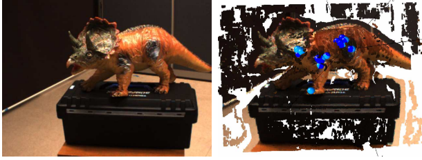
Fig. 8. Left : The left eye's image of figure 7's scenery. Right : The pose of the object is successfully determined using Rigid Motion minimization.
