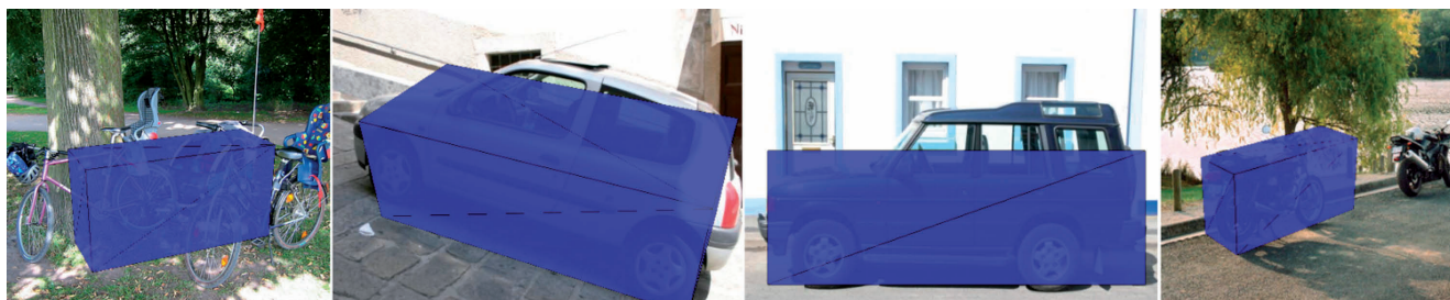
Figure 9. Remaining issues illustrated on a few examples from the PASCAL 06 dataset (from left to right): incorrect feature matches, failed 3D pose estimation, unknown object geometry, not enough features for a successful pose estimation due to the size of the objects. This figure is best viewed in color.
