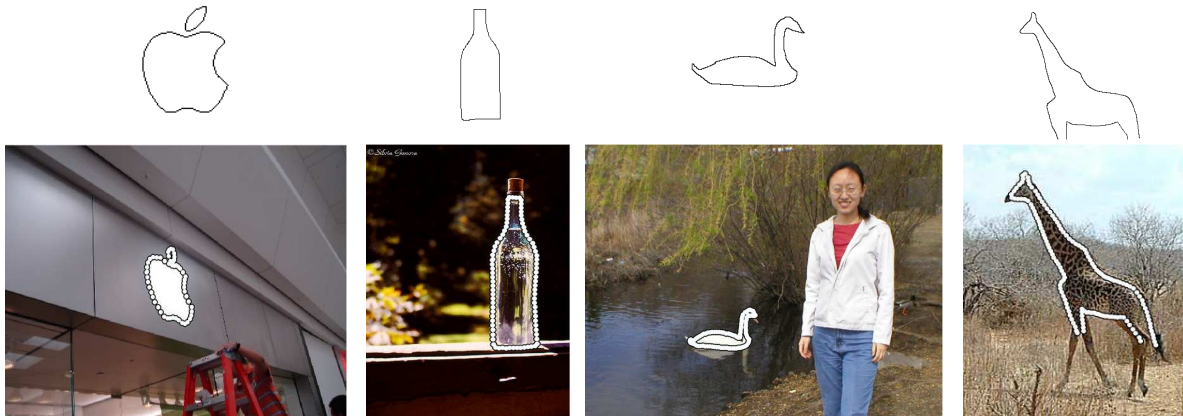
Fig. 18 Detection from hand-drawn models. Top: four of the five models from [14]. There is just one example per object class. Bottom: example detections delivered by our shape matching procedure, using these hand-drawings as models.
