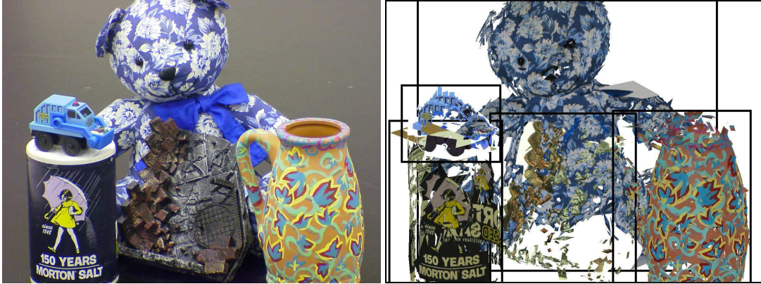
Figure 1. Results of a recognition experiment. Left: A test image. Right: Instances of five models (a teddy bear, a doll stand, a salt can, a toy truck and a vase) have been recognized, and the models are rendered in the poses estimated by our program. Bounding boxes for the reprojections are shown as black rectangles.
