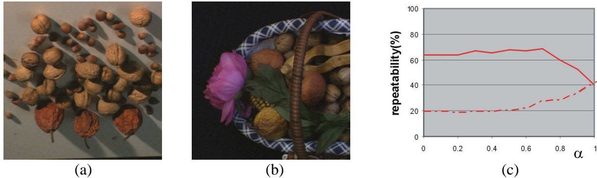
Fig. 5. (a), (b) Two frames from two sequences with changing illumination conditions. (c) Repeatability as a function of the amount of color saliency boosting. Dotted line for the sequence (a) and the continuous line for sequence (b).
