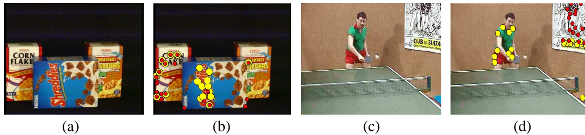
Fig. 2. (a) Example Soil data set and (c) frame from table-tennis sequence. (b) and (d) results of Harris detector (red dots) and the Harris detector with color boosting (yellow dots). The red dots mainly coincide with black and white events, while the yellow dots are focussed on colorful points.
