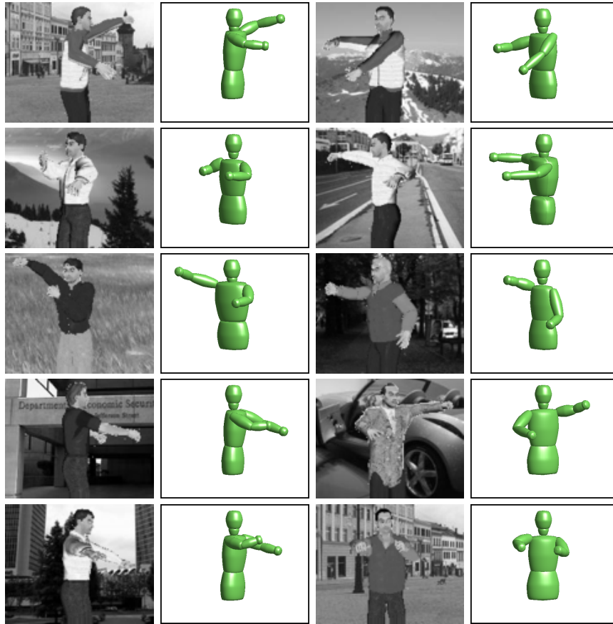
Fig. 5. Sample pose estimates from a test set of 1000 images in cluttered backgrounds. No knowledge of segmentation is used in the process.
