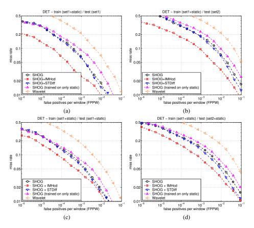
**Fig. 6.** An overview of the performance of our various detectors. All detectors are trained on *Training Set 1* combined with the *Static Training Set* with flow set to zero. They are tested respectively on: (a) *Test Set 1*; (b) *Test Set 2*; (c) *Test Set 1* plus the *Static Test Set*; (d) *Test Set 2* plus the *Static Test Set*.
