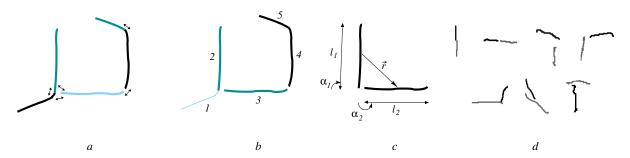
Figure 2. (a) Contour segment network edgel-chains connected at endpoints and junctions. (b) PAS = groups of two connected contour segments. (c) 5D PAS descriptor: orientations, relative lengths and location. (d) PAS codebook.
