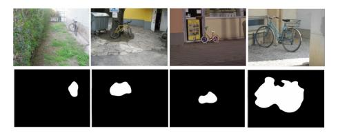
Figure 16. Binary segmentation masks for the bike category produced by the proposed method, see text.
