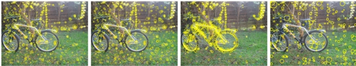
Figure 4. Examples of different sampling methods. (1) Harris-Laplace (HL) with a large detection threshold. (2) HL with threshold zero – note that the sampling is still quite sparse. (3) Laplacian-of-Gaussian. (4) Random sampling
