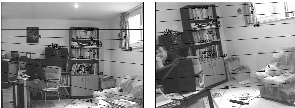
Figure 12: This figure shows the epipolar geometry as computed with the matching and estimation method described in this paper. Notice the large discrepancy in the viewpoints associated with the two images. The matcher seems to give advantage to collections of coplanar points.
